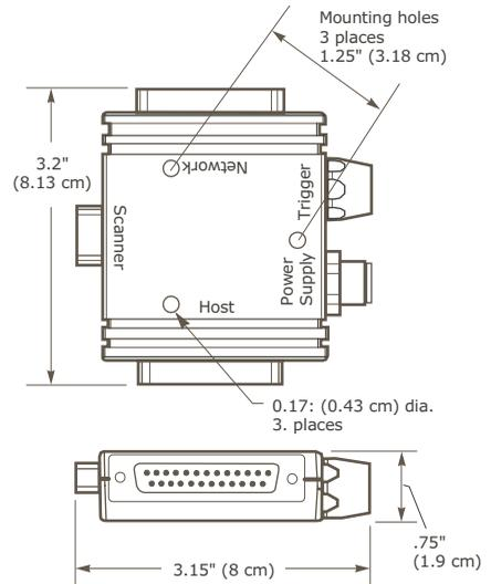
Figure A-7 IB-131 Mechanical
