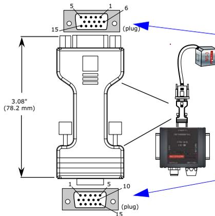
"READER" connector to MS-3 (with fixed nuts). See [Figure A-5, IC-332 READER Pinouts](#)
